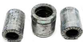
Samples after 720h tested according to ISO 9227 NSS
