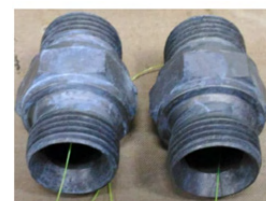
Samples after 720h tested according to ISO 9227 NSS
