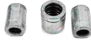
Samples after 400h tested according to ISO 9227 NSS
