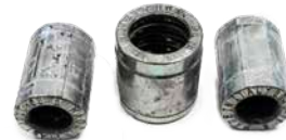
Samples after 720h tested according to ISO 9227 NSS
